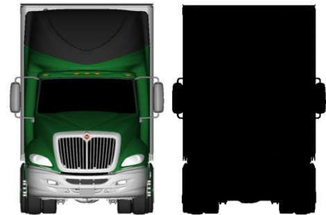
Figure 31 Width Based Reference Area for a Navistar ProStar with Van Trailer
