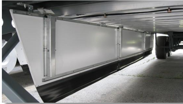
Figure 46 Ground Clearance Precaution with Aero Performance (Wabash)
