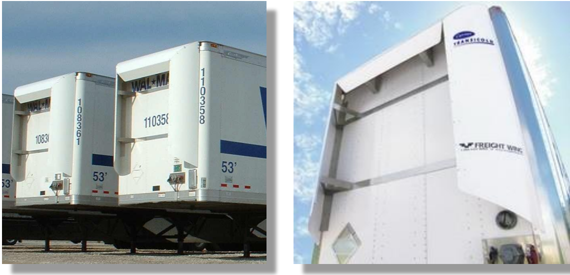
Figure 58 FreightWing/Carrier Gap Devices
