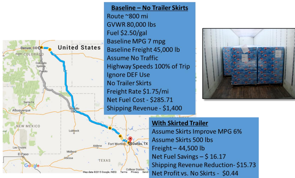
Figure 24 Beverage Hauler Aero vs. Weight Evaluation
