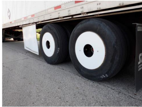
Figure 61 Solus Wheel Cavity Cover
