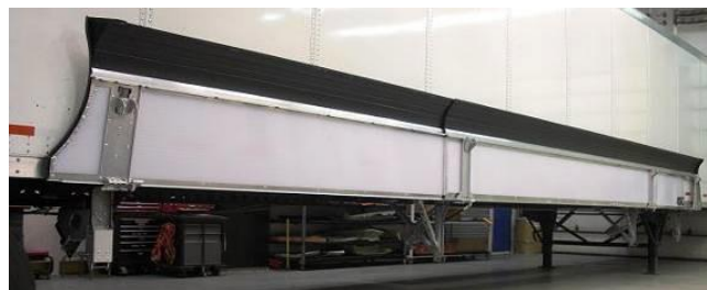
Figure 47 Articulated Skirts Allow Clearance at the Yard (Windyne)
