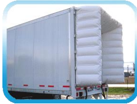
Figure 55 ATS SmartTail Inflatable Rear Aero System (ATS)
