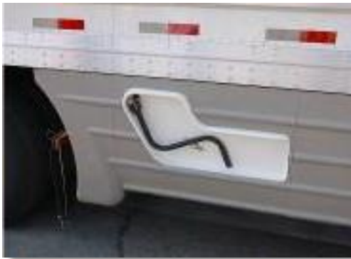
Figure 41 Formed Skirts (Laydon)
