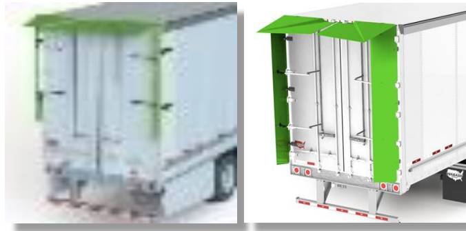
Figure 52 Wabash AeroFin and AeroFin XL Rear Aero Devices (Wabash)
