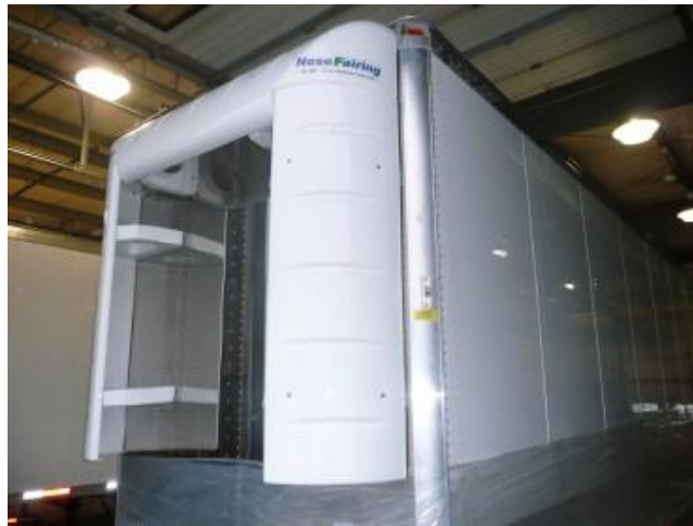
Figure 57 Nose Fairing Gap System (Laydon)
