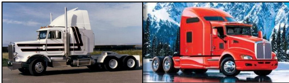
Figure 23Aero Design Integration from Discrete Fairing and Sleeper to Integral Aero Sleeper
