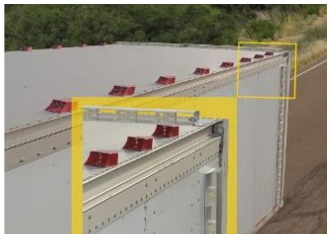
Figure 68 VorBlade Wing System
