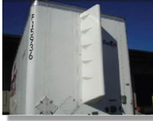
Figure 60 Vortex Stabilizer Device (Laydon)
