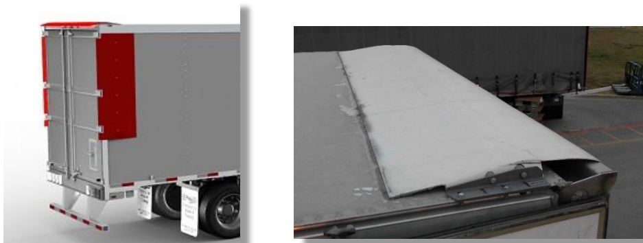
Figure 53 TopKit Trailer Tail System (SmartTruck)
