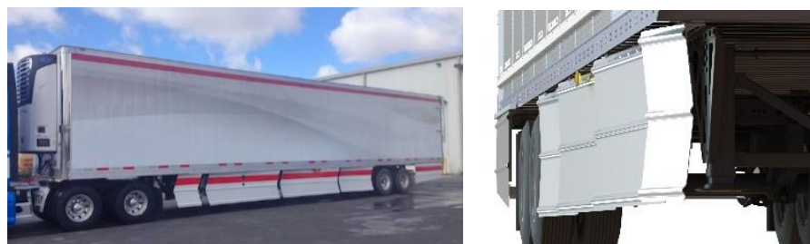
Figure 45 Segmented Skirt Aerodynamic Devices (Wabash)
