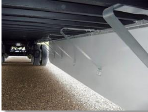
Figure 40 Example Skirt Installation (Utility Trailer)
