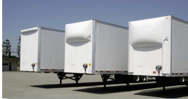
Figure 56 NoseCone Trailer/Tractor Gap Devices
