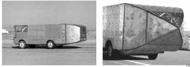
Figure 48 Trailer End Design Getting to the Point (NASA)
